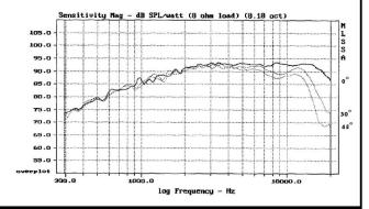
Measured on IEC baffle using Bruel & Kjaer 3144 model microphone. Also available in black faceplate finish.
